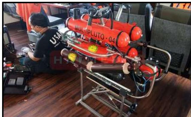
Gambar 2.32. Remoted Operational Vehicle (ROV)
